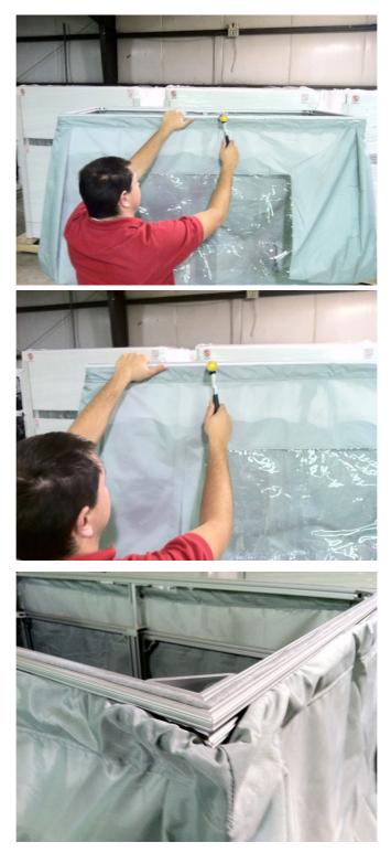
15 The bottom frame rail has 3 grooves. Fabric is to be placed in the top groove. If the lower grooves are used, then the zipper door will not work properly.
