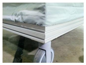
17. Repeat step 14. Start in the centers of each side and secure corded fabric into top groove of bottom rail. Repeat halving the distance between each section until entire perimeter of fabric is securely in the groove.
