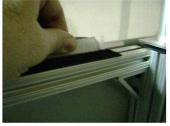
8. Separate the hook from the loop of the Velcro. Loosen fabric so it can be removed.
