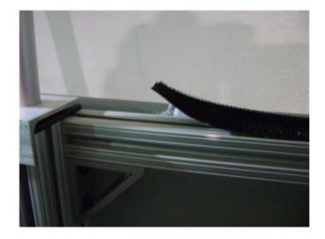
Page 7 of 23 DUZcart.com 888-389-2278 v5.0 9. The easiest way to remove the cover is to simply cut the entire length of fabric from top to bottom at either cart end. Discard cover upon completion.
