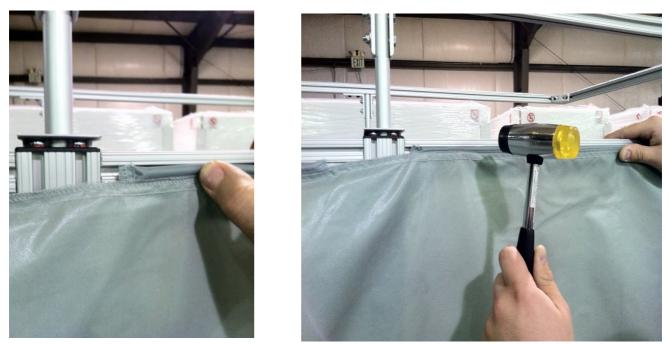
12. Work the top portion of the fabric to the upper moveable carriage. Verify that all of the corners are aligned.
