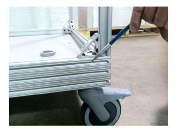
16. Align and tap corners first on bottom rail. (This is a repeat of the top carriage fabric installation).
