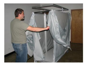
11. Take time to vacuum and clean the base and frame. Standard household cleaner and a dry cloth works well. If the floor has become scuffed, a light abrasive cleaner such as Soft Scrub or Magic Eraser does a good job at removing scuffs.
