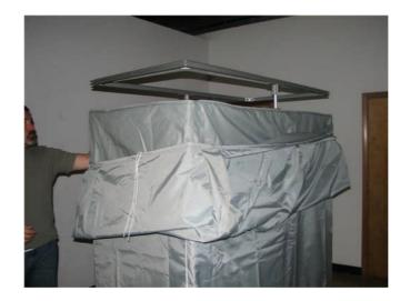
Page 17 of 23 DUZcart.com 888-389-2278 v5.0 11. Align corded fabric into position and lightly tap into place with a mallet. Corded pouch should tap securely into frame along entire length. Excessive force is not required and will damage the fabric. Repeat on all sides.
