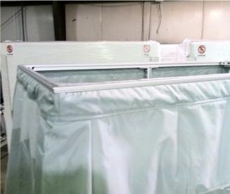
19. Upon cover installation, test the up and down motion of the upper carriage.
