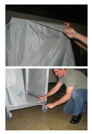
2. Remove all cabling at top and bottom perimeter of cart.
